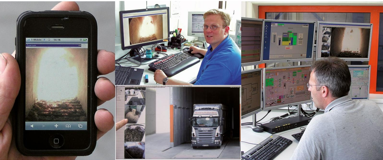
the lens is blown clean again with a compressed air nozzle. And this camera, protected by a dust-proof housing, plays the part perfectly. Another camera on top of the chimney monitors the color and the quantity of the smoke produced. On clear days, it stares directly into the sun for hours without generating burning effects or forming streaks. Cameras with CCD sensors don't have what it takes to stand up to these harsh conditions.
