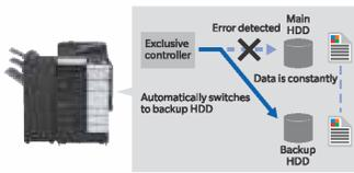
This feature ensures that all data saved on the main HDD is always saved on a backup HDD as well. If the main HDD fails, bizhub C759/C659 automatically switches to the backup HDD to prevent operational downtime and data loss.
