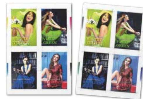
CMYK and RGB+gray(3C) are alternately printed on the margin of the printed sheets. In addition, registration marks are automatically printed on both sides of the sheet to check registration.
