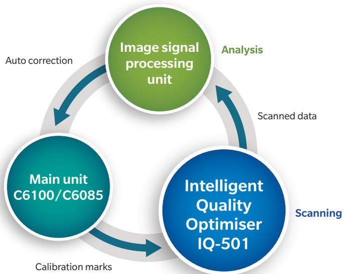
Accurate colour and registration adjustments are performed in a single pass that includes automatic printing, scanning and analysis of front-to-back registration marks and gradient bars.
