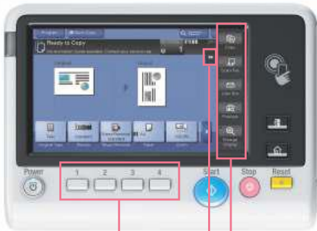
Hard registration keys Register up to 4 commonly used function.
